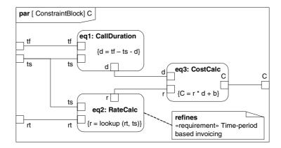
**Fig. 3.** Parametric diagram for billing feature (simplified) in model of [4], to support analysis and identification of input parameters that must be made available by a domain architecture to support implementation of a requirement for time-period based call invoicing
