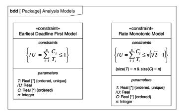
Fig. 4. Reusable analysis models for hard-real time system families packaged as constraint blocks
